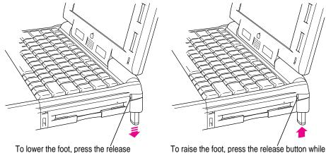
To lower the foot, press the rélease button. The foot extends automatically.
